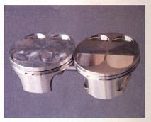
The new piston and the old one. The new version is bigger, but weighs less and is expected to last about three times as long.
