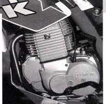
An 8mm smaller piston makes the 605 into a 494. The carb is 2mm smaller. Although the crank and rod are the same, the 490 vibrates much less than the 605.
