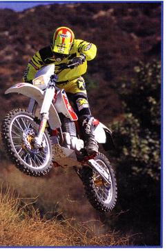
Even the smallest jump bottoms the Paioli fork, as it falls through the travel quickly with stock settings. The PDS shock isn't as soft as the fork. For moto, crank in the compression clickers at both ends.
