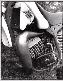
Also during the late '80s, ATK offered its first two-stroke models. Unlike ATK's four-strokes, the rotary-valve 250 and reed-valve 406 weren't the horsepower kings of their classes, but their air-cooled, non-power-valved engines and linkageless rear suspensions appealed to riders who were put off by complex machines.
