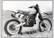
'87. Some of the first ATKs were built around Honda engines to test the company's unusual countershaft disc brake and anti-chain torque device. Many ATKs were sold as frame kits. Engine supply problems led ATK's founder to strike a deal with Austrian engine builder Rotax.
