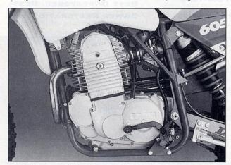
A time-proven, air-cooled Rotax motor puts out smooth and linear power, with tons of torque on tap. This is the same four-valve motor that is used on most 600cc dirt-trackers.
