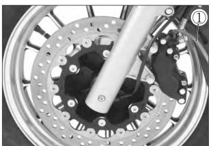
■ Loosen the air bleeder valve and pump the brake lever until the old brake fluid is completely out of the brake system.
