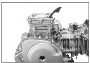
Remove the rear cylinder head and cylinder with the same manner of the front cylinder head and cylinder removal.
