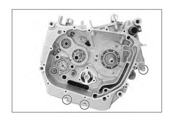
Remove the mission oil pipe mounting bolt.
