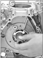
■ Apply the SUPER GREASE "A" to the driveshaft Oring and oil seal lip.
