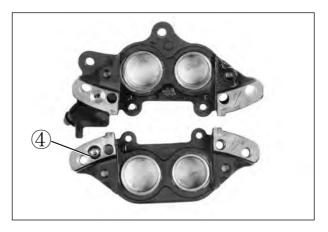
• Using compressed air, push out the caliper pistons.
