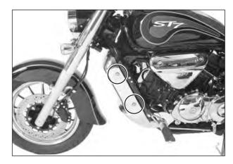
Remove the four radiator mounting bolts.
