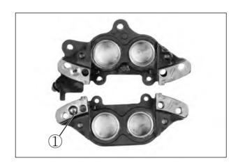
■ Tighten the caliper housing bolts ② to the specified torque.
