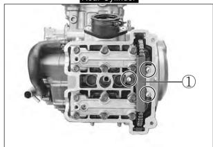
$\bullet$  Remove the camshaft housing 2.
