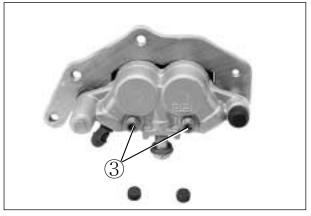
• Remove the brake pad mounting bolt 3.
