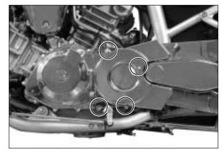
With the four mounting bolts, remove the drive belt cover.
