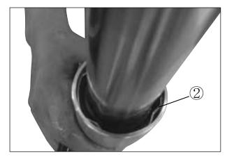
Remove the oil seal ③ and oil seal retainer ④ by using the special tool.
