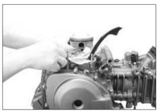
• Remove the piston pin by using the special tool.
