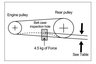
Recheck the drive belt slack after tightening the rear axle bolt.
