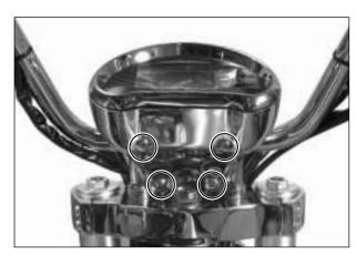
With the instrument panel bracket mounting bolts removed, remove the instrument panel.
