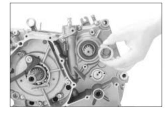
Install the oil seal retainer.
