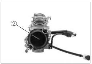
■ Remove the spring ① along with diaphragm ②.
