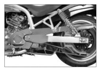
With the rear shock absorber lower bolts removed, disconnect the rear shock absorber from swingarm.
