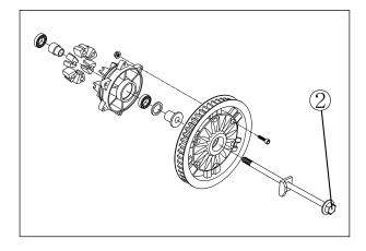
With the disk mounting bolts removed, remove the rear brake disk cover and brake disk.
