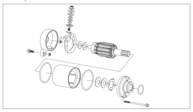
● Align the mark ① on the housing with the line ② on the housing end.
