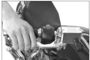
Squeeze and release the brake lever several times in rapid succession and sqeeze the lever fully without releasing it. Loosen the bleeder valve by turning it a quarter of a turn so that the brake fluid runs into the receptacle, this will remove the tension of the brake lever causing it to touch the handlebar grip. Then, close the air bleeder valve, pump and squeeze the brake lever, and open the valve. Repeat this process until the fluid flowing into the receptacle no longer contains air bubbles.
