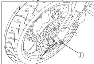
● Tighten the front axle bolt ① and axle pinch bolt ② to the specified torque.
