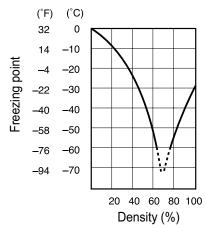
Fig.1 Engine coolant density-freezing point curve.
