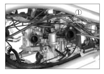
• Remove the engine ground lead wire ①.
