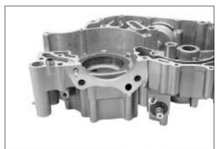
$\bullet$  Install the oil jet 1 to the oil hole of crankcase.
