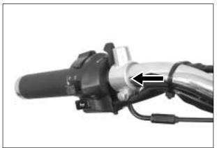
Apply SUPER GREASE "A" to the throttle cables.
