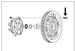
With the rear wheel installed, tighten the rear axle bolt ① to the specified torque.
