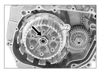
With the clutch sleeve hub held immovable using special tool, remove the clutch sleeve hub nut.
