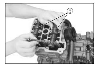
Loosen the cylinder head base bolt.
