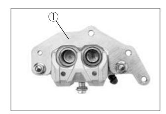
• Using an air gun, push out the caliper piston.
