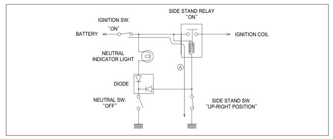
"Aguila" is equipped with the side stand ignition interlock system.
