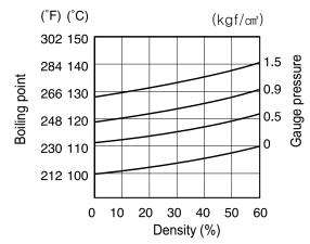
Fig.2 Engine coolant density-boiling point curve.
