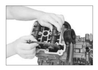
The "1F" arrow of exhaust camshaft sprocket should be toward the outside and aligned with the plane of FRONT cylinder head.
