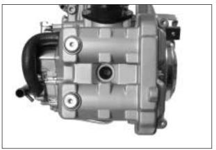
Install the rear cylinder head and cylinder with the same manner which installed the front cylinder head and cylinder.
