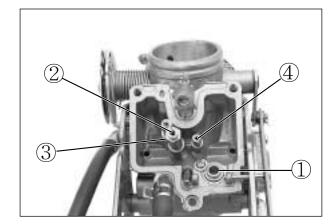
■ Remove the pilot screw ⑤ counting and tightening the number of turn.
