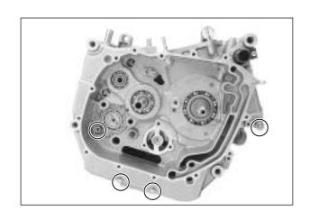
• Remove the mission oil pipe mounting bolt.
