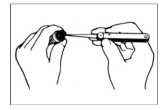
Check to see the worn or burnt condition of the electrodes.
