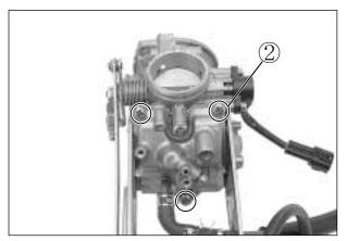
Align the hole ① of the diaphragm with passage way on the carburetor body.
