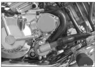
Remove the snap ring and water pump driven gear
