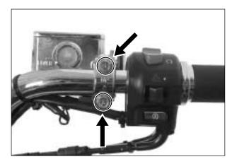
Remove the two fitting screws and separate the cap and diaphragm.
