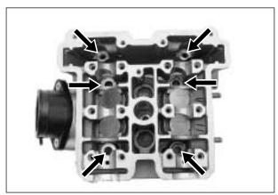
■ Remove the chain guide NO.1 and cylinder head.
