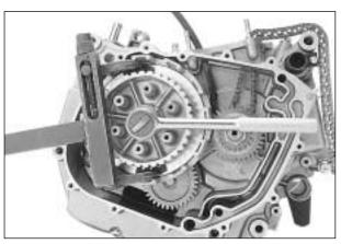
Remove the clutch sleeve hub ① and primary driven gear assembly ②.
