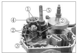
Remove the crankshaft by using the special tool.
