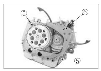
Install the clutch cover, and tighten the clutch cover bolts securely.
