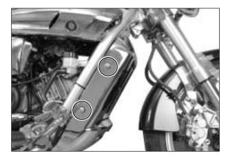
Remove the four radiator mounting bolts.
