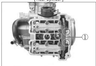
$\bullet$  Remove the camshaft housing  $@\ .$
