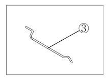
Lift the rear end of the fuel tank and prop it up as shown illustration.
