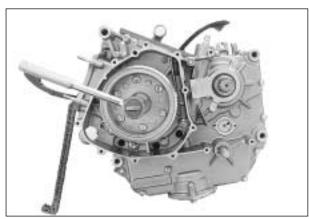
Remove the magneto rotor by using the special tool.
