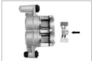
Apply SILICONE GREASE to the brake caliper holder.
