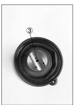
Align the hole 4 of the diaphragm with passage way on the carburetor body.
