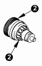
Ocheck both gears Ø for wear.Othe starter gear has to grip exactly in one direction.
