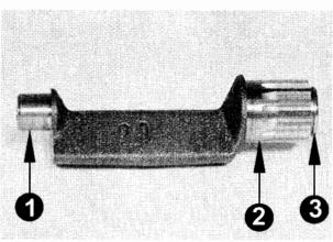
Balance shaft, balance drive gears
