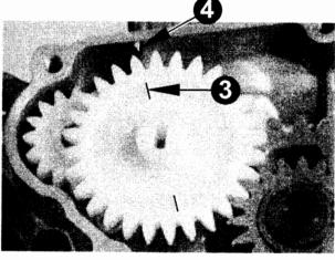
Put idle gear (3) on axle and align with mark (4) on crankcase by turning of the crankshaft.
