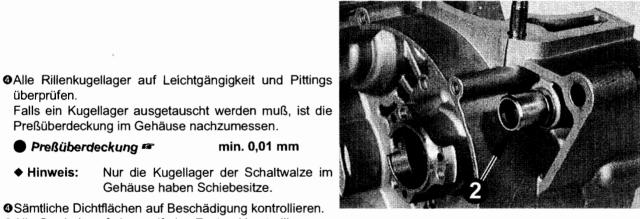
Ocheck all ball bearings for easy motion and pitting. At the renewal of a ball bearing check the press fit in the crankcase.
