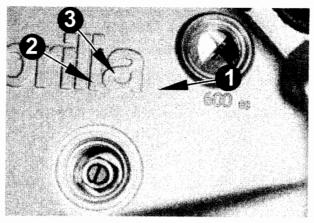
Attach combustion chamber insert **1** with 5 hex. hd. screws M8 **2** and lockwashers.
